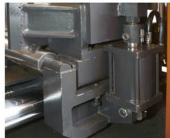
Floating Cylinder to Prevent Material Friction with Front Vise.
