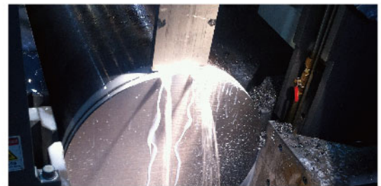
Automatic centering compact coolant supply unit is able to cool cutting area directly. (Patented)
